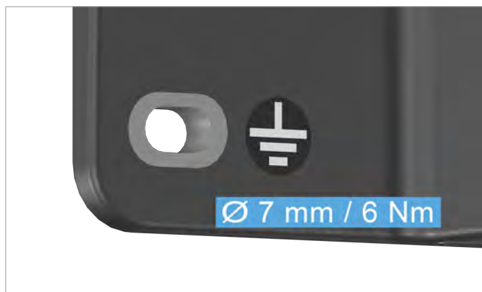
Fig. 5.15: Grounding connection at the left mounting hole
