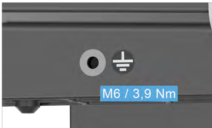
Fig. 5.14: Grounding screw on the left foot of the inverter
